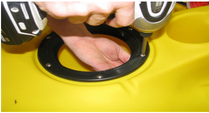
Fig.#II Install Hatch
